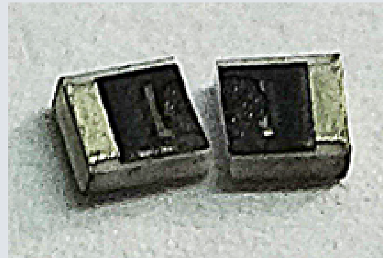
Y司抗浪涌 1206 CHIP型电阻 (100Ω、5%)
